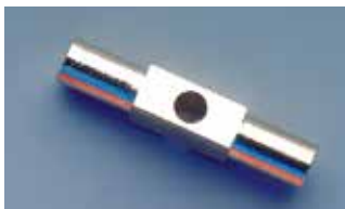
SFC/CO Cat. No. FC102 Ø 6,3 x 32 mm - in brass for terminal block types: FPC.10 - SFC.10 - SFR.6 - with possible derivation by means of plug SDD/2
